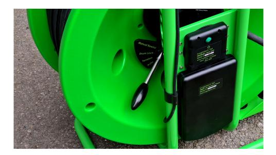
The only external difference between the manual and auto drums is the addition of the control lever as seen above. But hidden in the centre of the hub is a three-phase brushless motor and Troglotech-designed Cycloid gearbox providing enough power to retrieve 300m of cable and the crawler at 0.5M/S
