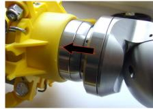
Tighten camera onto the T804 camera termination
