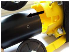
Ensure that the T804 camera termination is free of water or debris, clean if required. It is imperative that the slipring area is clean and free from moisture.
