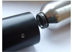
Slide the T804 camera termination and the internal adaptor tube into the skid.
