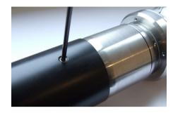
Unscrew camera from T804 termination and internal adaptor tube.
