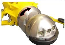
Lightly tighten 3 x Allen screws onto the camera body. Do not over-tighten these screws as this may distort the camera body
