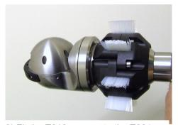
3) Fit the T812 camera to the T804 termination
