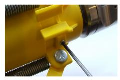
Set the skid to the correct diameter for the pipe being surveyed and then lightly tighten the friction bolts to hold the skid in position. For pipes between 150mm-200mm, use the small wheel set.
