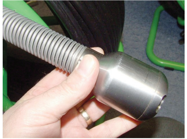
2) Fit camera to Rod Termination
