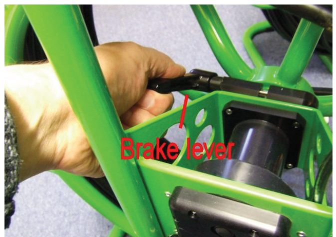
6) Adjust the brake to supply a small amount of friction. You are now ready for surveying
