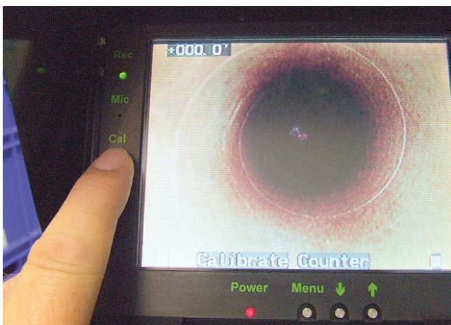
5) Press the Rod Counter button until the display shows 'Counter Calibrated'
