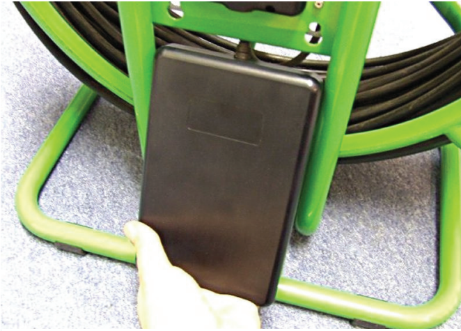
1) Slot Power Cell into frame and push upwards to lock in place
