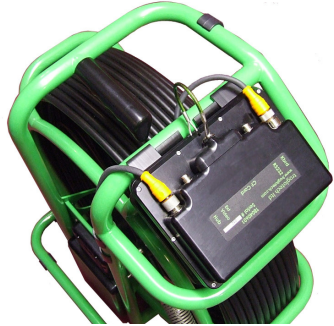
2) Fold the sunshade flat, swivel Control Unit flat against keyboard
